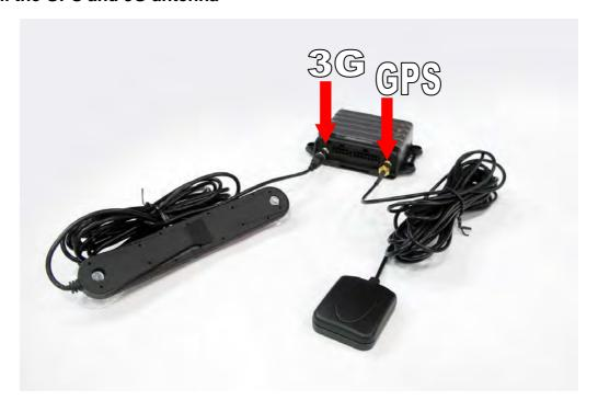
Install the 3G antenna to the 3G antenna port on the left side of the front of the device. Install the GPS antenna to the GPS antenna port on the right side of the front of the device.
